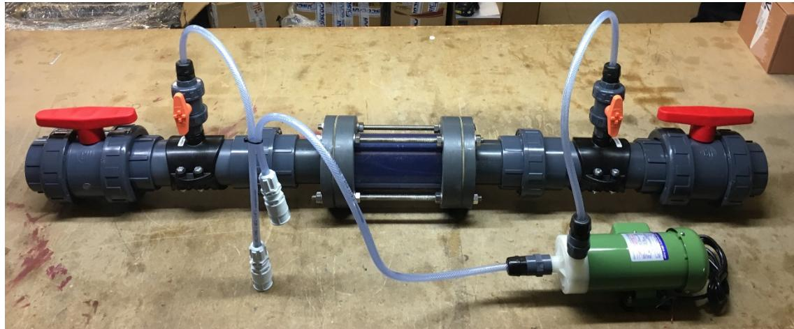
Once installed, stop filtration and close the inlet and outlet valves of the cell
