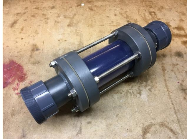
Fit half of the connector with the cap and pour cleaning fluid into the cell. Wait for a few minutes, remove the cleaning fluid, examine the state of the cell and repeat the procedure if necessary.
