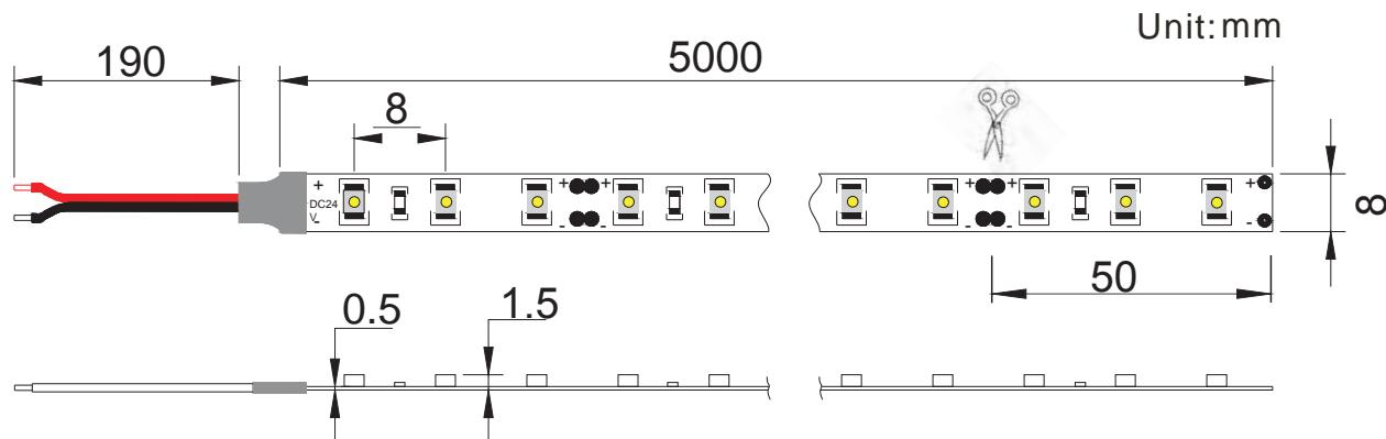
ESQUEMA DE CONEXION MONOCOLOR / SINGLE-COLOR CIRCUIT DIAGRAM
